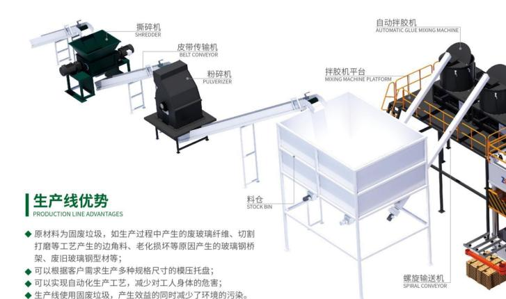
The raw materials are solid waste, such as waste glass fibers generated during the production process, scraps produced by cutting and polishing processes, fiberglass bridge frames and waste fiberglass profiles caused by aging and damage, etc; We can produce molded trays of various specifications and sizes according to customer needs; It can achieve automated production processes and reduce the harm to workers' health;
