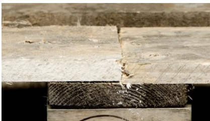
The general condition is so poor that the safe working load is obviously no longer guaranteed (e.g. rotten, decayed boards/blocks, or boards / blocks comprising several pieces).
