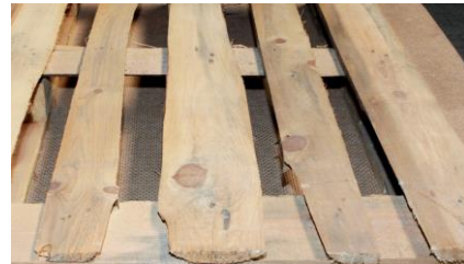
Boards / blocks with incorrect dimensions or made of unapproved material.
