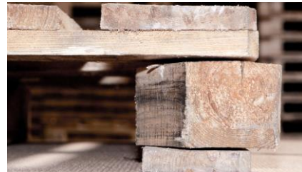
One or more blocks are twisted so that one corner of the block protrudes more than 1 cm above the outer edge of the pallet.
