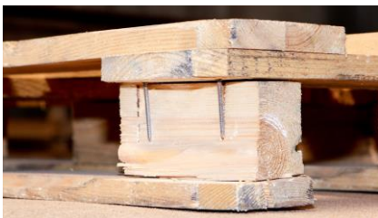
One or more blocks are split in such a way that more than one nail shank is visible.
