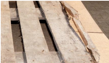
One or more boards are broken crossways or at an angle, or split in such a way that more than one nail shank is visible.
