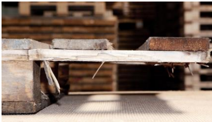
One or more boards / blocks are missing in part or in full.
